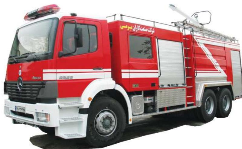
**Water pump:** output :4500-6500 lit/min ,10 bar.
