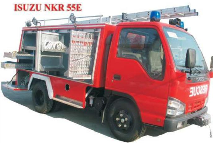
Solid compartment by special forming sheet and all shelves and storages are equipped with three position hinges aluminium shutters are used to store tools and other equipment , All the shutters are equipped with safety locks and all the lights are fixed in their proper position .
